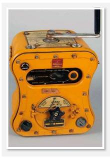
**Model / Maker:** Made in six versions, BC-778-A/F, differing only in details of electrical or mechanical design.
