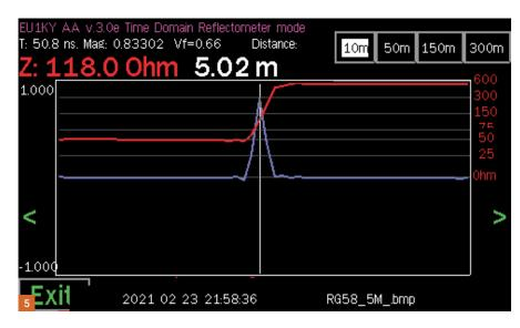
For this to work correctly, the Velocity Factor (Vf) of the cable must be known and entered into the unit. The unit is pre-set with a value of 0.66 (such as for RG58). This may be altered and stored, either temporarily or permanently. I found this feature accurate although; with some cables, the analyser presented some odd impedance values directly at the cut-off point (Fig. 5).
