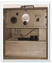
Battery-operated 2-valve transmitter/receiver. **Transmitter:** Output 0.3w, R/T only. **Frequency coverage:** 44.0 to 61Mc/s.
